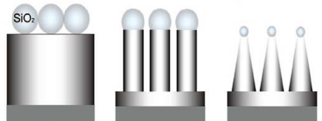
Fig. 1. Fabrication Process of Nanowires and Nanocones
